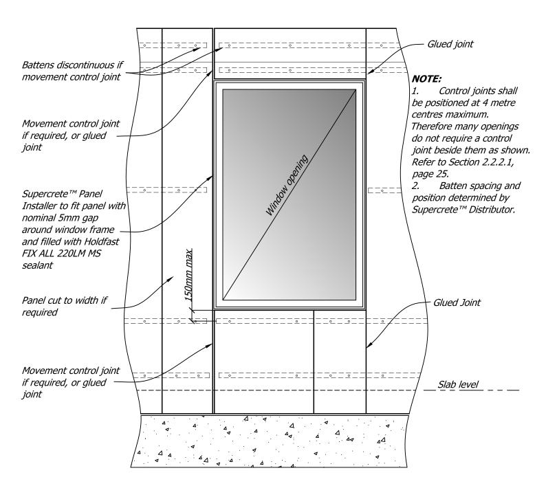
Steelock™a unique steel top hat batten mounting system.
